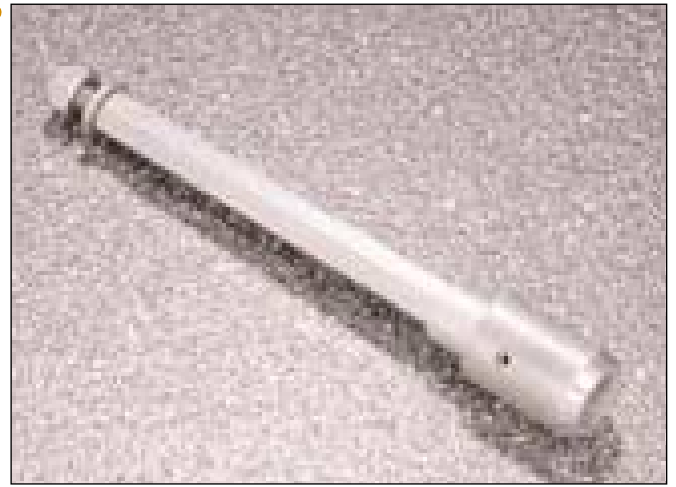
Pressed & Pinned Shaft/Coupling Assembly
